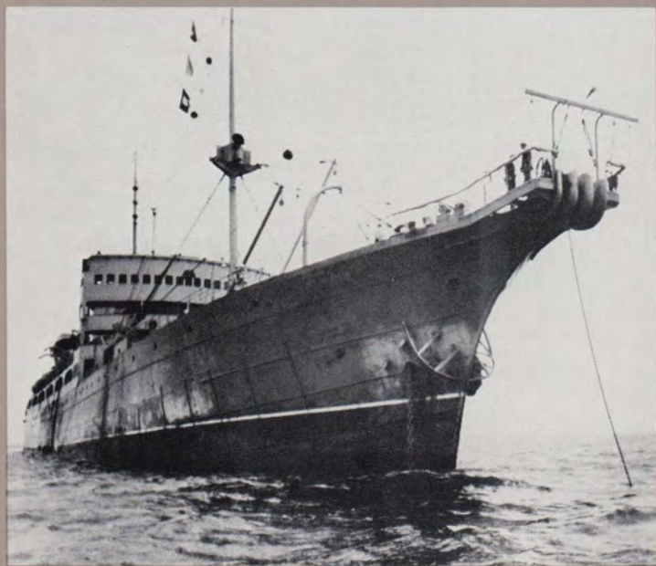
This ship, H.M.T.S. Monarch , laid the first trans-Atlantic telephone cable. The first telegraph cable had been laid by the Great Eastern in 1866 and radio-telephony had been commercial since 1927, but the first telephone cable came in 1956. Many others followed. Our newest will be lightguide.
