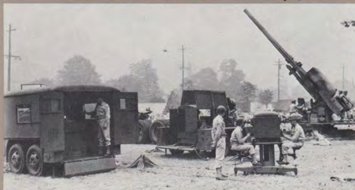
The Western Electric M-10 electrical gun director, which continuously and automatically set fuses on shells and aimed this 120 mm anti-aircraft gun.
