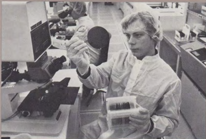
Left—The incorporation of integrated circuits in many of our switching and transmission products necessitated the building of clean rooms in our factories—facilities often cleaner than the operating room of a hospital. This one is at the Allentown Works.
